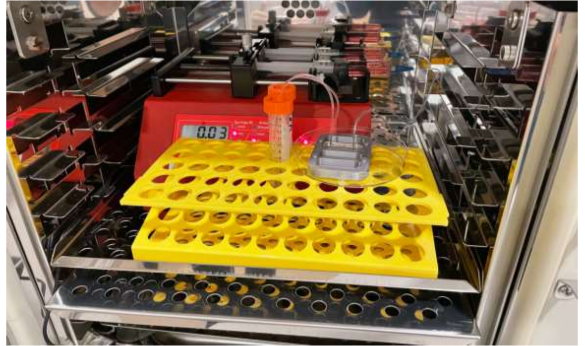
Incubator setup (chip, chip tray, perfusion pump, connectors, and output vials)
